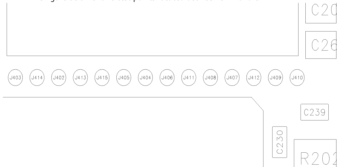
Figure 8: Test points Located Between UEM and UPP.
